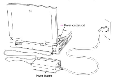
A lightning bolt icon appears in the battery monitor portion of the Control Strip when the power adapter is plugged in and a battery is recharging.
